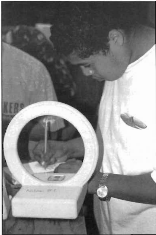
Above--STEP's Christopher Swimptkin jots down data taken from fish scanner. Halo-like device checks PIT tag from fish. Below--Dirk 'D.J.' Spencer uses elbow grease to sweep bottom of fishway. Photos by Carol Craig.
