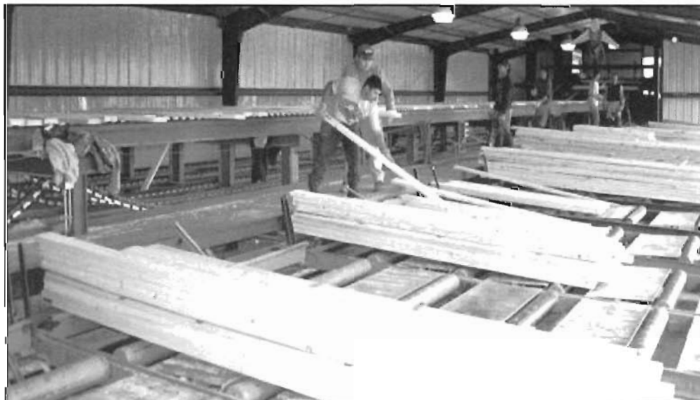
The final stage of cutting, employees sort the different sizes into stacks to be dried and packaged.
